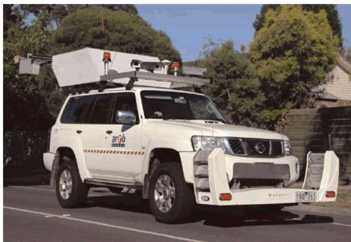
Figure 2.1: Network survey vehicle (NSV)
