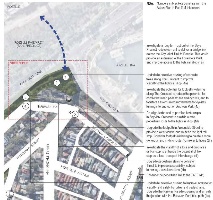
FIGURE 13: RECOMMENDATIONS - BURUWAN PARK AND ROZELLE BAY LIGHT RAIL STOP (not to scale)
