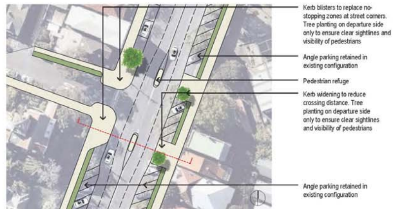
FIGURE 20: TYPICAL PLAN STREETScape TYPE 3 - KERB WIDENING AT INTERSECTIONS (not to scale)
