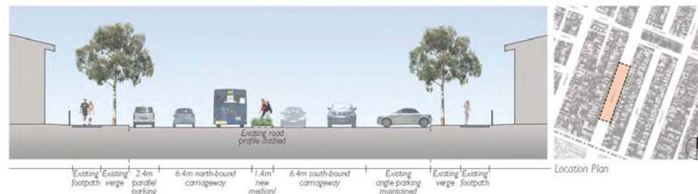
FIGURE 18: TYPICAL SECTION STREETScape TYPE 2 - PARALLEL PARKING AND ANGLE PARKING, 1:200 @A3
